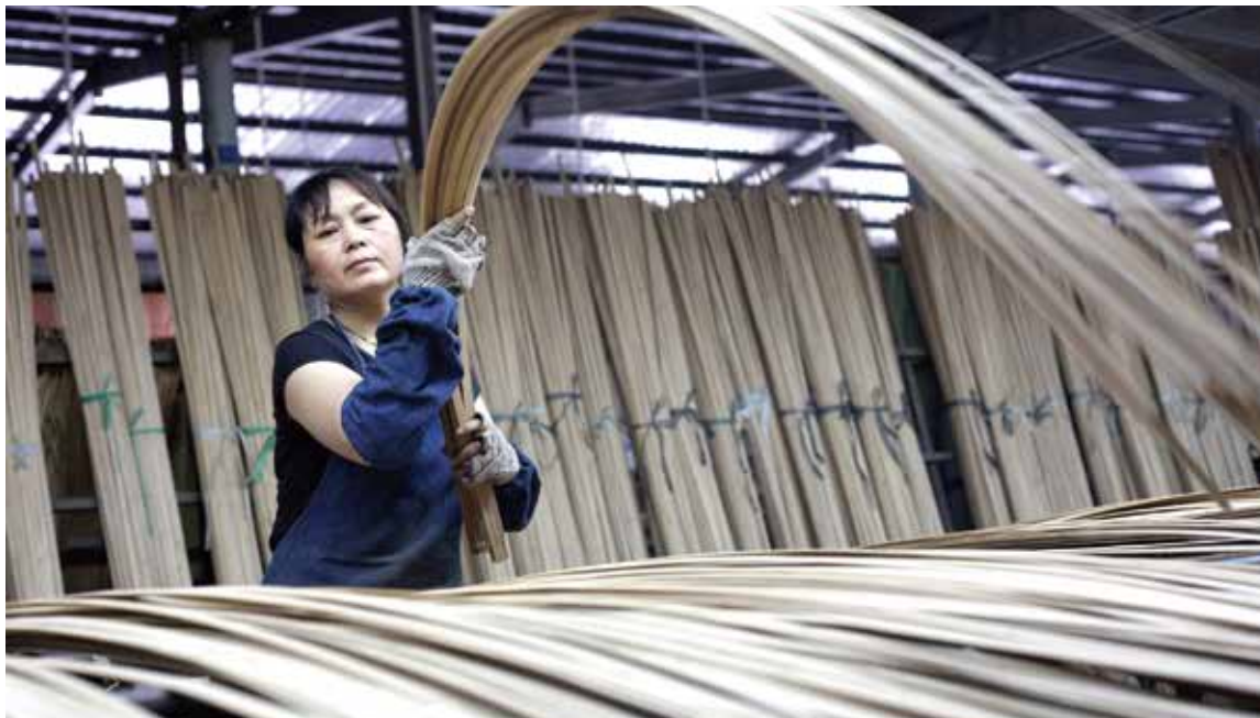
Bamboo splits are selected for pressing into boards at a factory in China
